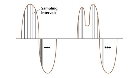
Realistically a brief glitch of 2 wrong 8 bit samples out of 8000 in the wave form as shown would show up as a click in the conversation which might not even be noticeable. Now suppose we throw in a delay equal to a three or four packets of more typical size of several hundred bytes each. Now we begin to approach a serious
