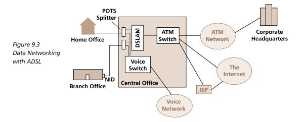
Although Figure 9.3 shows them as separate pieces, the central office POTS splitter may be a part of the DSLAM, and in some cases, all this hardware may actually be contained on the voice switch line card itself with the concentration of the traffic from many ADSL modems performed by a new common card in the switch line card shelf.
