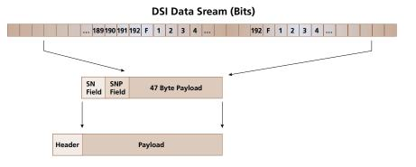
Note that the bits of the DS1 are streamed into the SAR PDU payload without regard to the framing of the DS1. The SAR PDU payload holds 376 bits which is just shy of two 193 bit DS1 frames.
