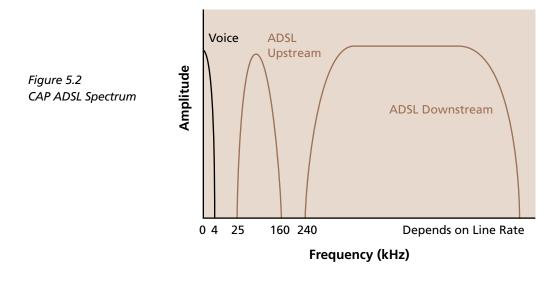
not necessary. Similarly, an echo from the user generated upstream channel is not a problem since the receiver is not listening in that range–don't need echo cancellers either. And since the frequency bands for transmit and receive don't coincide, NEXT is not a problem–you are not listening in the same place your next door neighbor's modem is transmitting.
